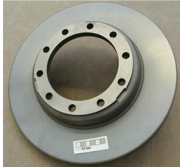
Figure 10. Titanium alloy truck brake rotor with a protective thermally-sprayed coating applied to the friction surfaces.
