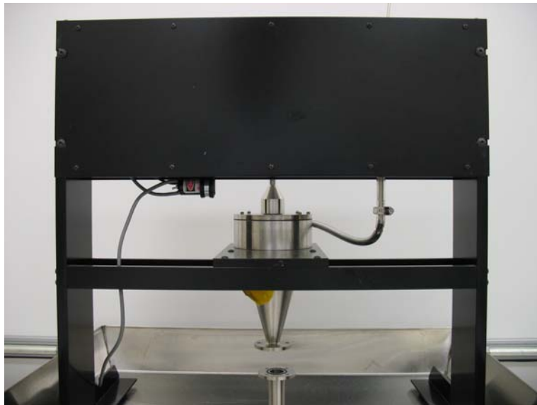
Figure 12. PSA as seen prior to operation with all panels in place. Cyclone separator is visible below enclosure.
