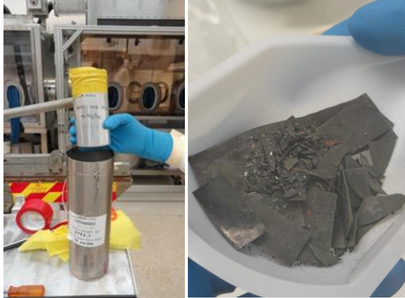
Fig. 2. Unpacking solid materials. Image at right shows some debris warranting segregation (brown brush hair, rusted pieces, white paper flecks, etc.).
