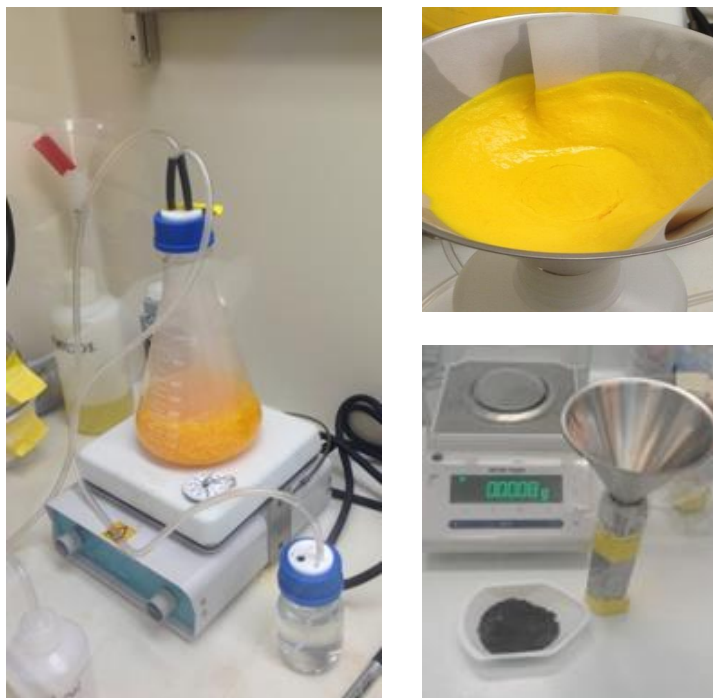
Fig. 4. High-purity ^{233}\text{U} precipitated as ammonium diuranate (left) and filtered (upper right). Lower right image shows calcined oxide, ready for loading into a bored-plug container (standing next to the oxide, with a funnel in place for filling).
