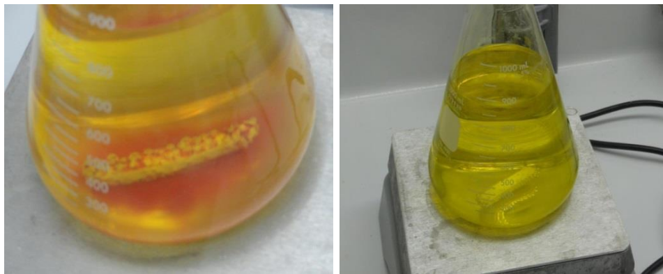
Fig. 3. High purity ^{233}\text{U} being dissolved (left) and completely dissolved (right). [A magnetic stirring bar can be seen in the bottom of flask in both images.]
