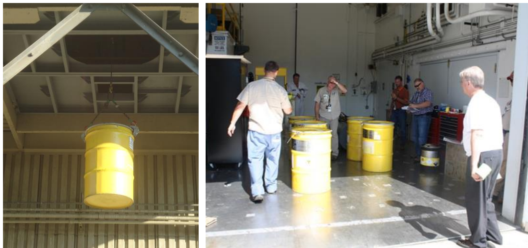
Fig. 1. Shipping drum containing high purity ^{233}\text{U} being removed from the repository (left image) and being received at an ORNL staging (temporary storage) facility (right image).
