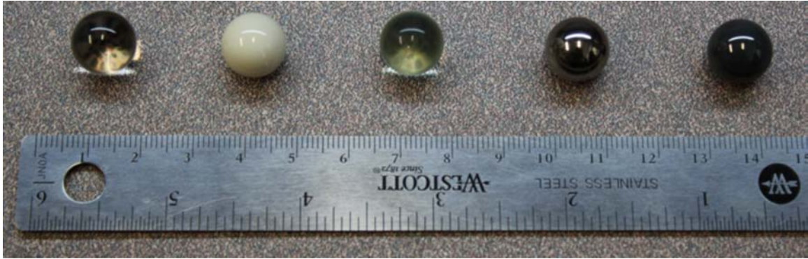
Figure 4. Spheres used for impact testing (from left to right): borosilicate (BS) glass, alumina ( \text{Al}_2\text{O}_3 ), soda-lime silicate (SLS) glass, steel, and silicon nitride ( \text{Si}_3\text{N}_4 ).
