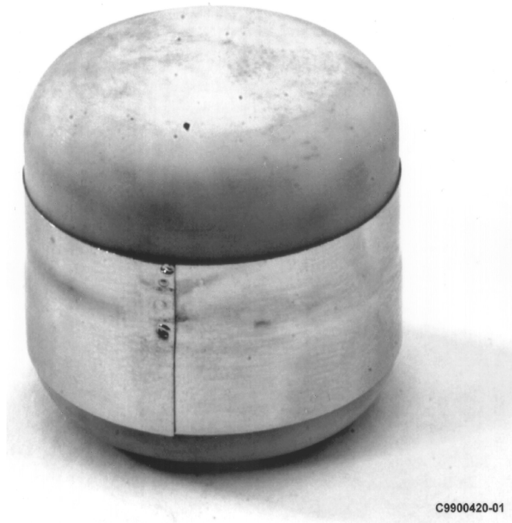
Fig. 23. Alumina simulant pellet with Type II shield laser welded tight around it.
