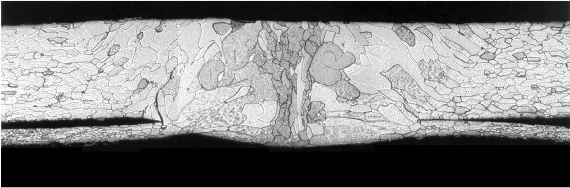
Fig. 21. Transverse cross section of a weld shield fusion (47×).
