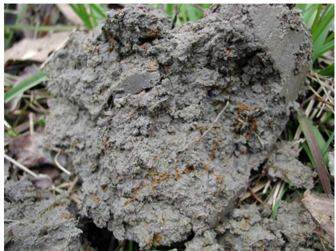
Fig. 8. Contrast between commonly encountered non-wetland soil (left) and wetland soil (right) surveyed within the Haul Road route. The strong gleying (right) is characteristic of sustained wet conditions. The orange streaks are oxidized rhizomes.
