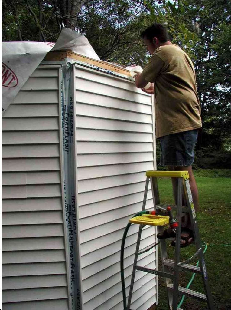
Fig. 10. Water being applied to top of panel.
