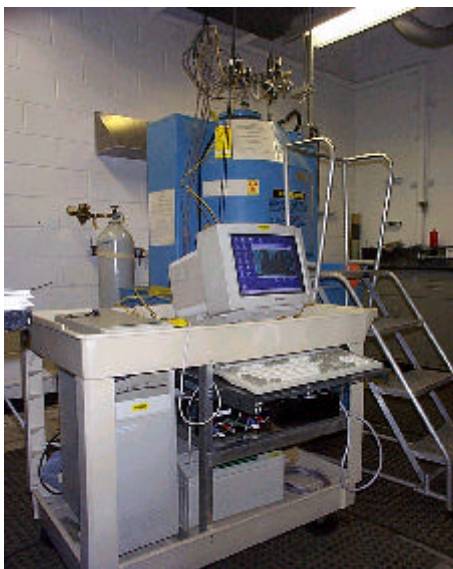
Fig. 2.5. Photograph of data acquisition computer in operation at the ORNL ^{60}\text{Co} source.
