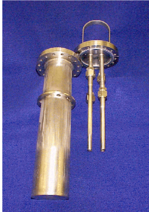
Fig. 2.11. Multiple-irradiation container used in HFIR SNF irradiations.
