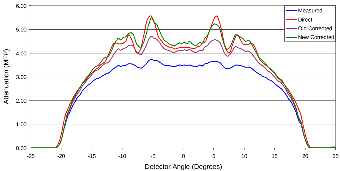
Fig. 7.36 Attenuation curves for the barrel measurement. Both the old and new (with empirical correction factor) corrected curves are shown for comparison.
