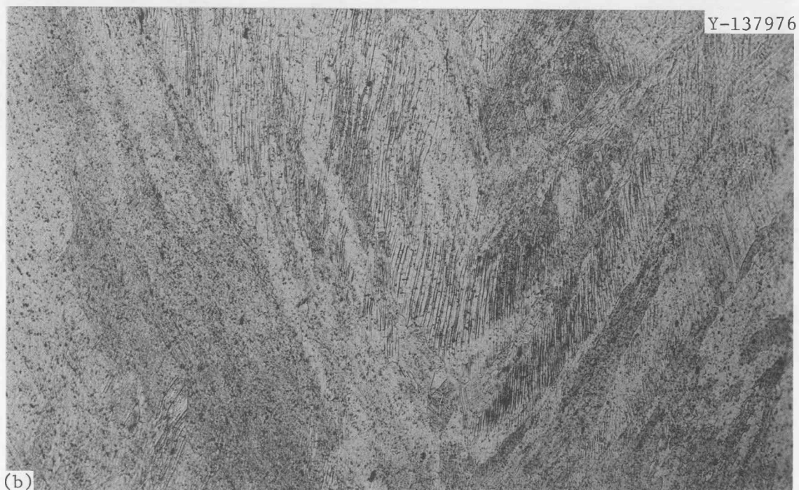
Fig. 4.11. Microstructure of Type 304 Stainless Steel Pipe Cold Worked 43.7%. 100 \times . Etchant: 50% HCl-10% HNO 3 . (a) Base metal. (b) Fusion zone.
