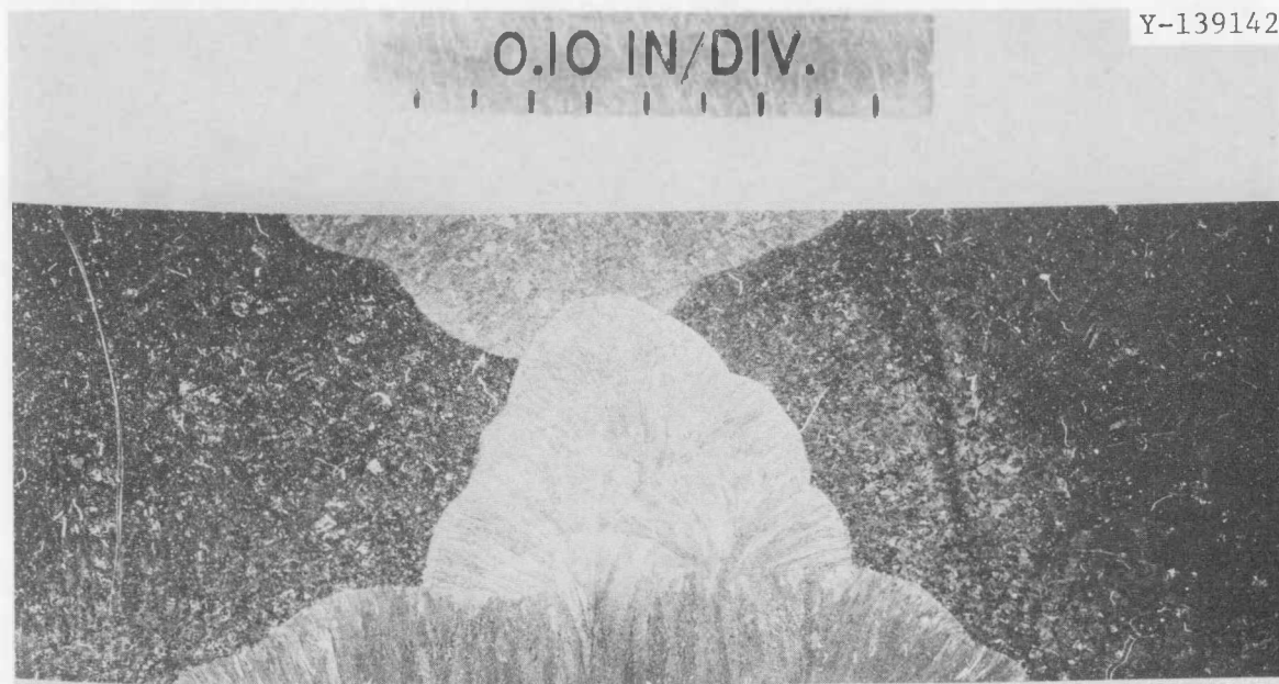
Fig. 4.5. Macrostructure of Type 304 Stainless Steel Pipe Cold Worked 20%. Etchant: 50% HCl-10% \text{HNO}_3 .
