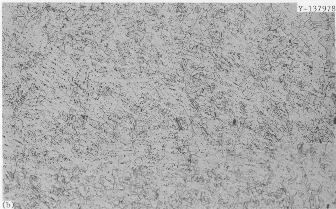
Fig. 4.12. Microstructure of Type 304 Stainless Steel Pipe Cold Worked 43.7% and Solution Annealed at 1066°C (1950°F). 100×. Etchant: 50% HCl-10% HNO 3 . (a) Base metal. (b) Fusion zone.
