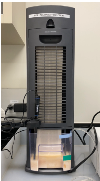
Figure 1. DAC setup using an Envion air humidifier as an air–liquid contactor.
