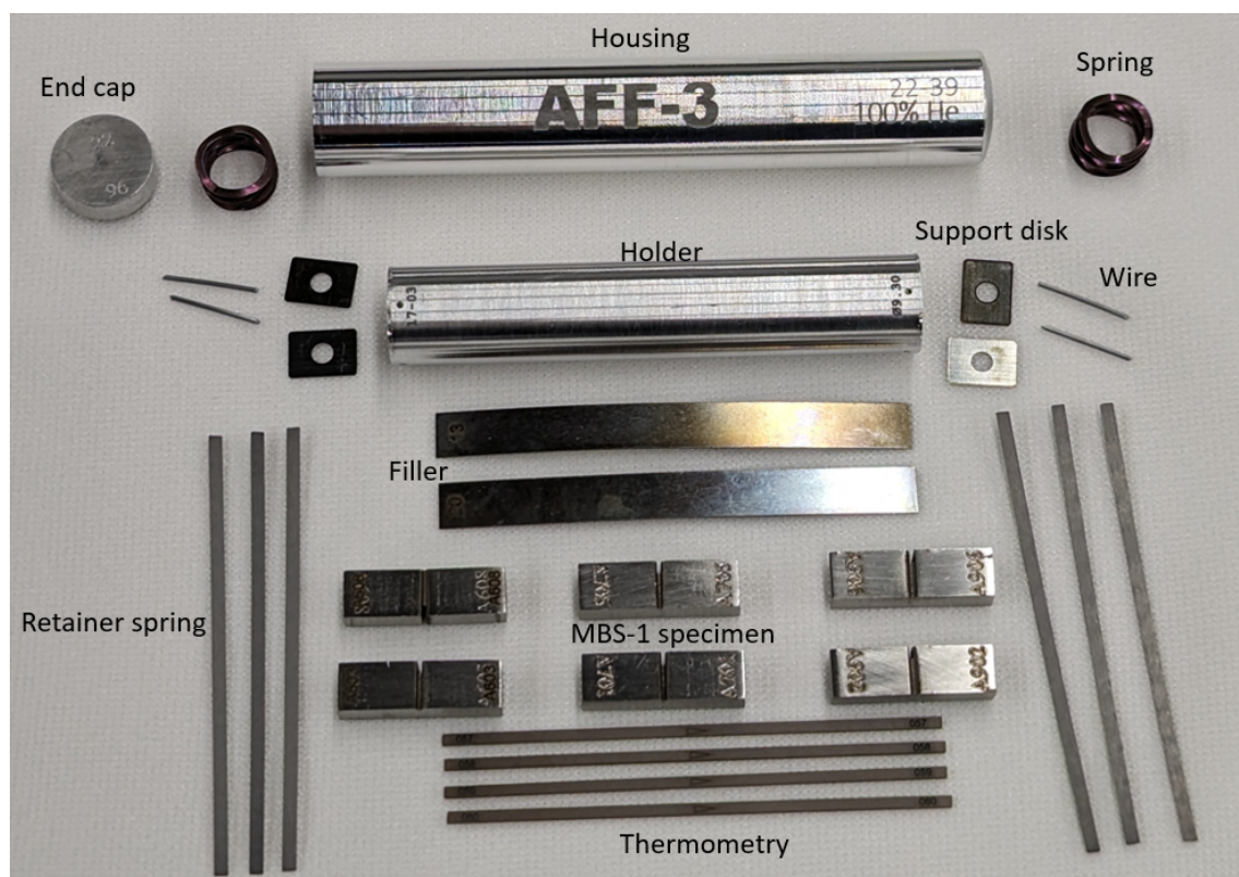
Figure 13. Example of MINBEN capsule parts layout.
