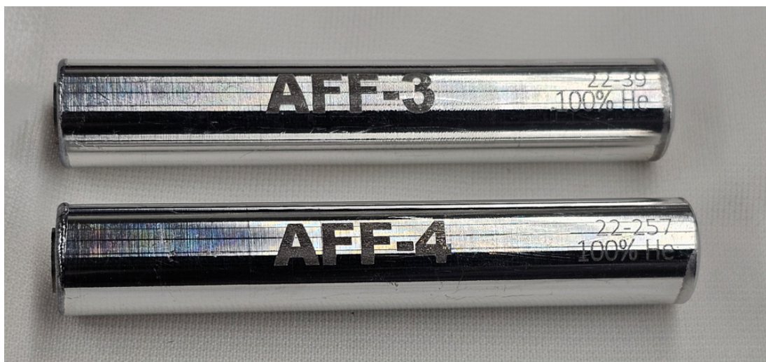
Figure 14. Capsules AFF-3 and AFF-4 fully assembled.
