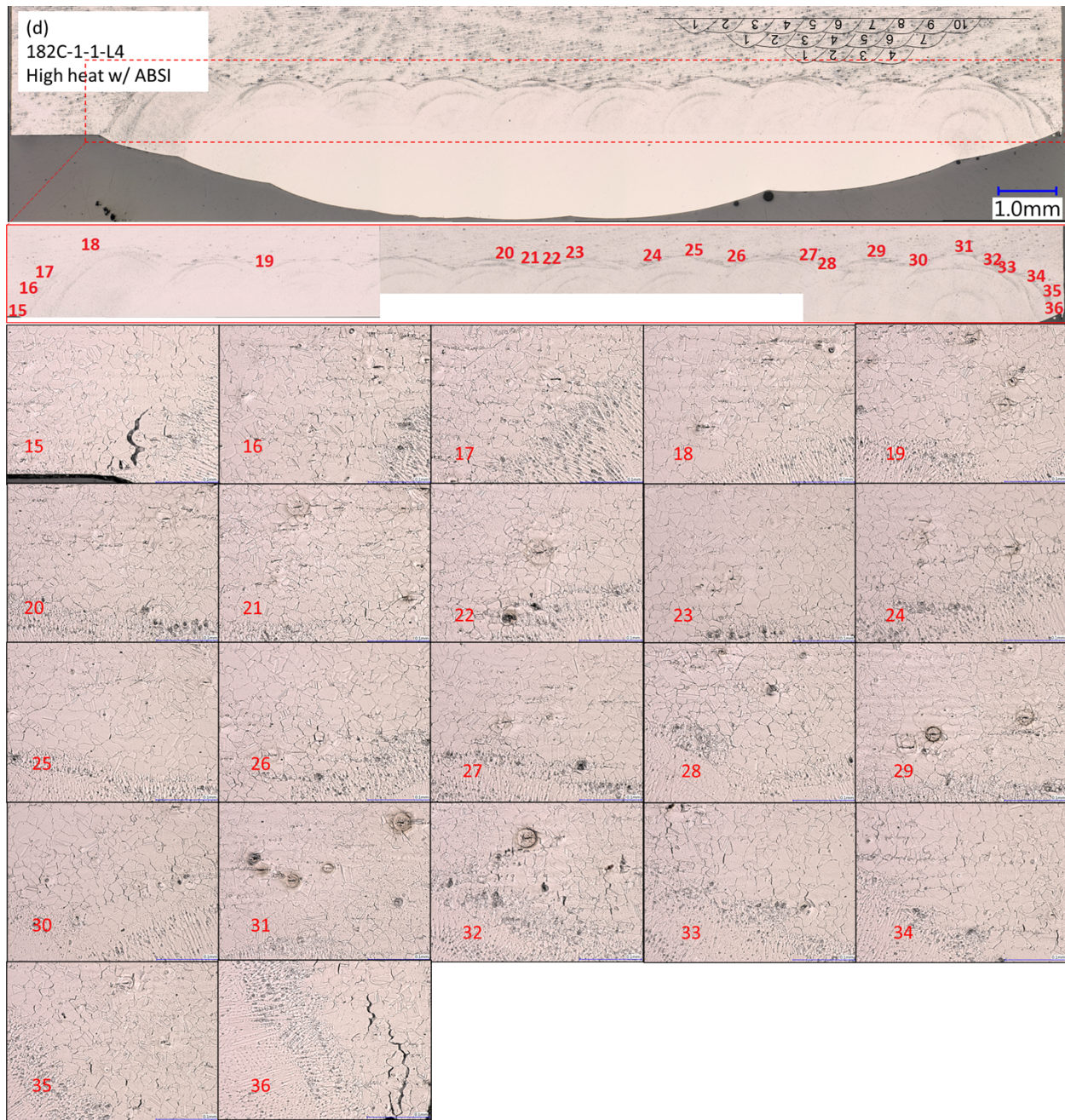
Figure 7 Cross-section views of LW cladding of alloy 182 with 15 wppm B with different welding conditions: (a) low heat input without ABSI; (b) low heat input with ABSI; (c) high heat input without ABSI; (d) high heat input with ABSI.
