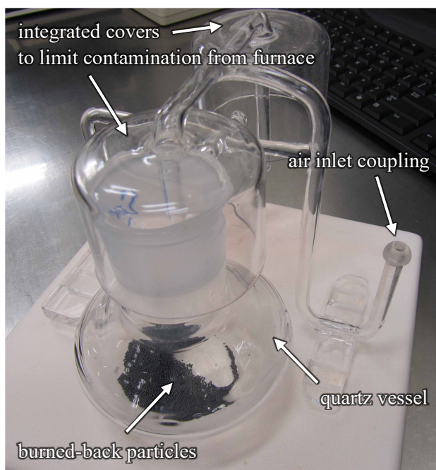
Figure 2-4. Two station covered air supply apparatus to facilitate the burn phase.
