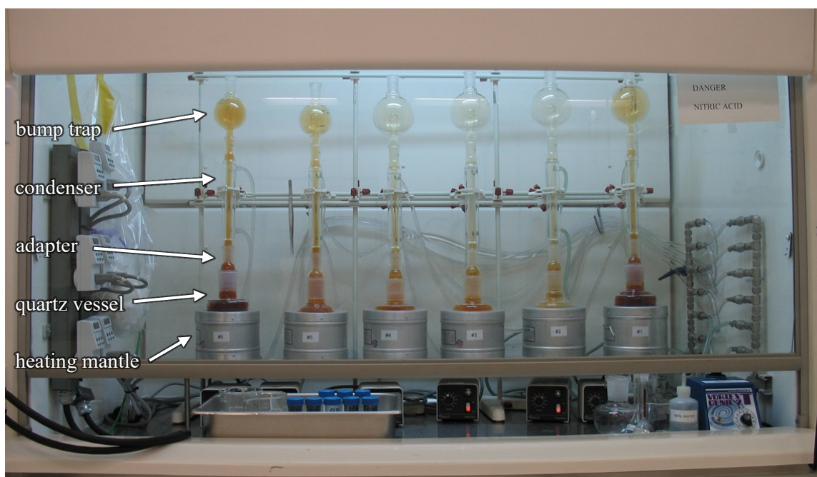
Figure 2-3. Leaching station showing six LBL reflux apparatuses.
