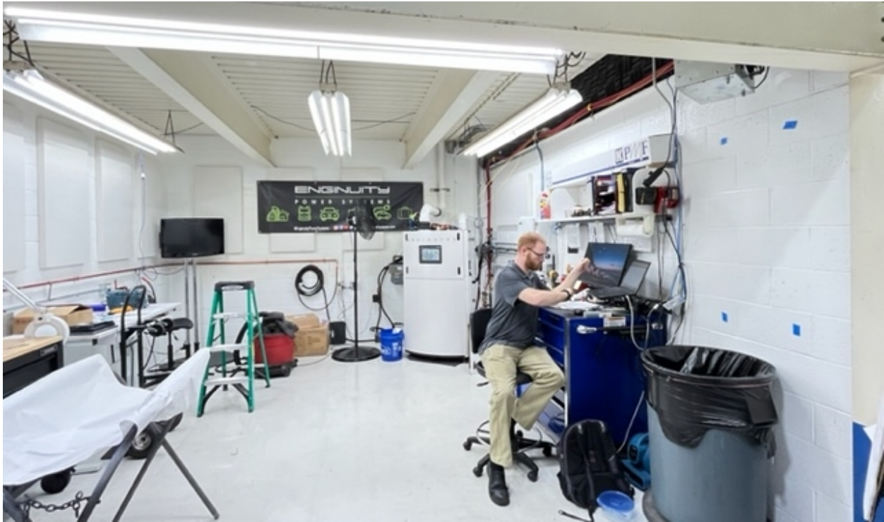
Figure 4: Enginuity's mCHP testing facility enabling electrical battery charging, water and space heating
