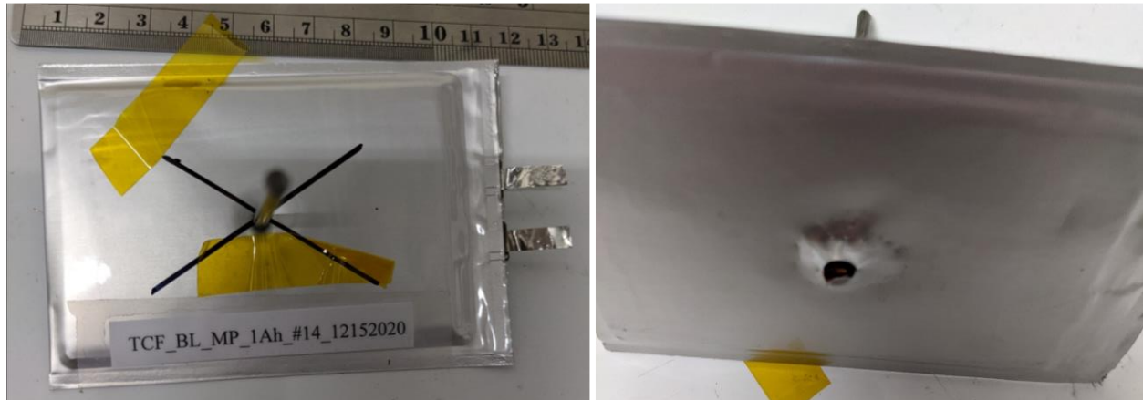
Figure 90. MP cell #14: top and bottom after testing (typical of all).
