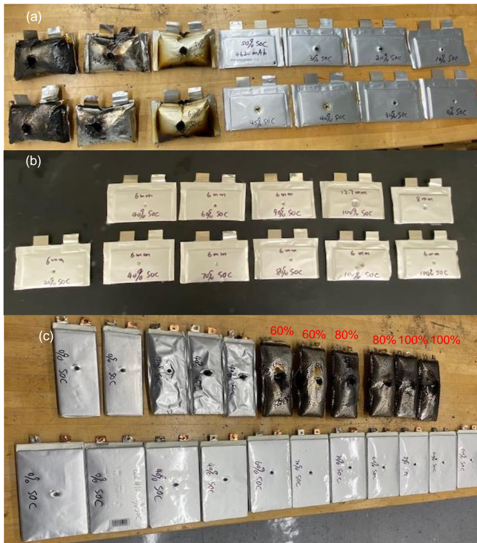
Figure 79. Cells after indentation testing: (a) control NMC 811 cells after testing, (b) MFCC NMC 811 cells, and (c) (top) 10 Ah NMC cells and (bottom) 10 Ah LFP cells.
