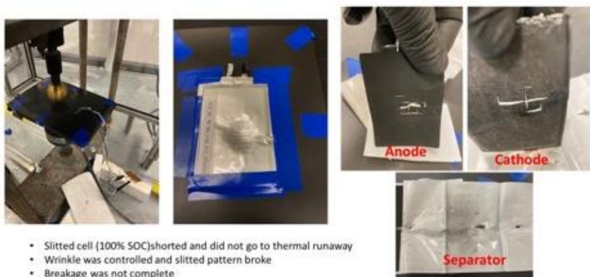
Figure 76. Using a closed Nissan Leaf top plate, and the slits opened up.
