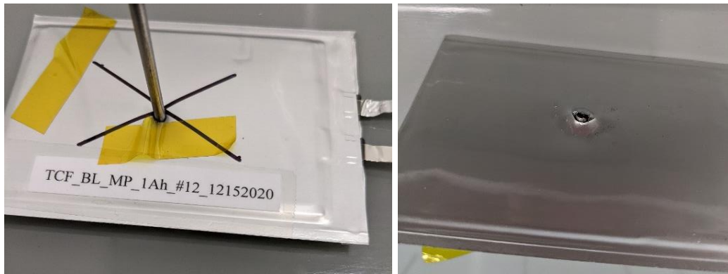
Figure 86. BL cell #12: top and bottom after testing (typical of all).
