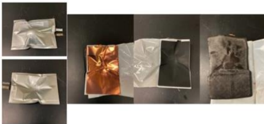
Figure 74. A slitted dry cell after indentation, and cell components.
