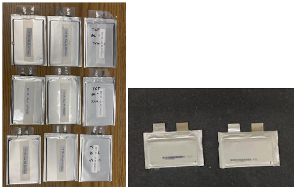
Figure 63. Baseline and slitted cells (1 Ah) received from ORNL’s BMF (left) and Soteria cells (5 Ah) (right).
