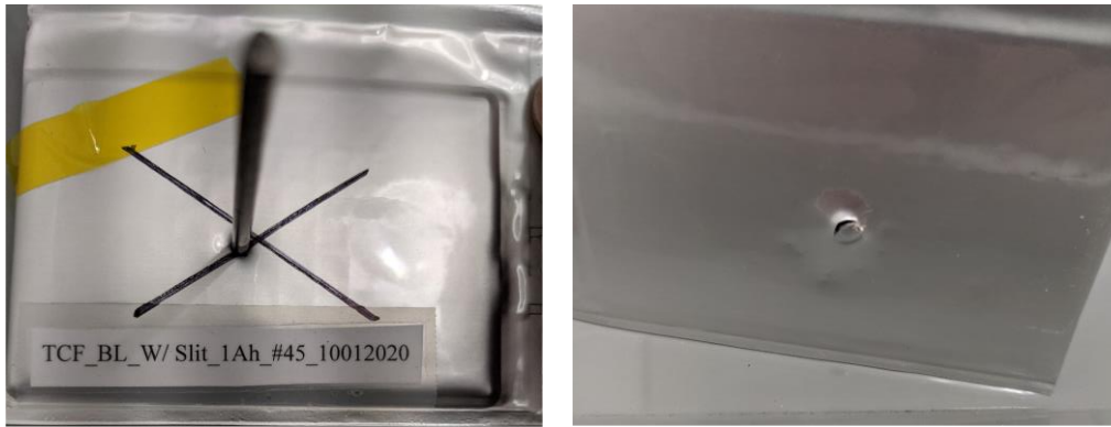
Figure 88. BL cell #45 with slits: top and bottom after testing (typical of all).
