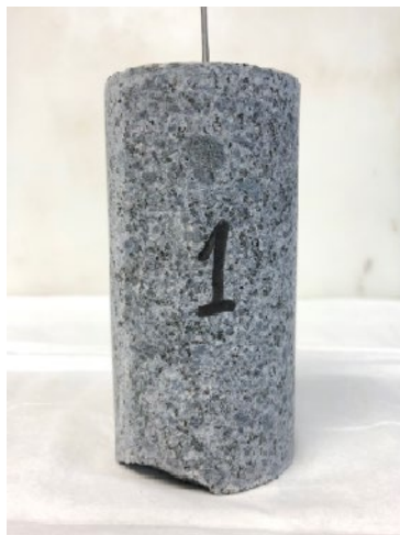
Figure 14 Image of tested specimen for g3001; no visible fracture on the surface of specimen after removed from the testing line.
