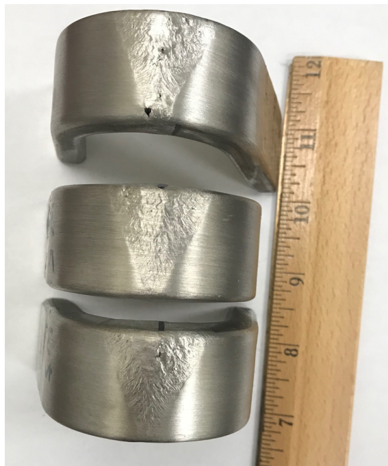
Figure 6. Side bend test results of Weld W5
