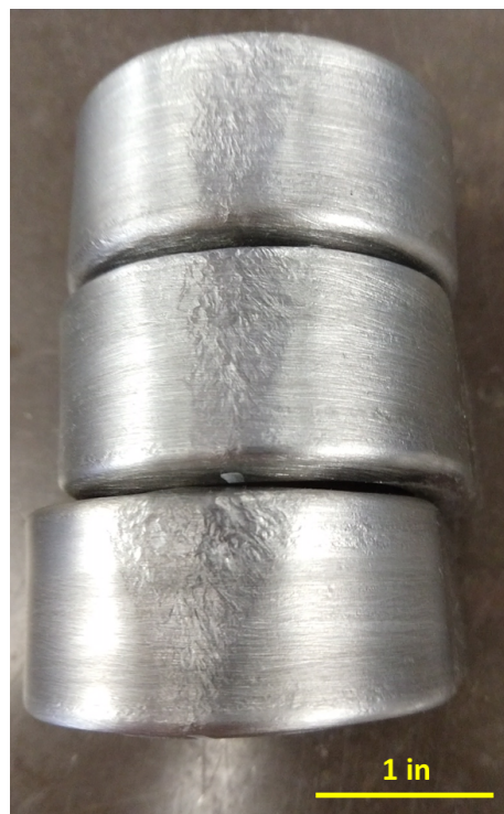
Figure 11. Side bend test results for Weld W6
