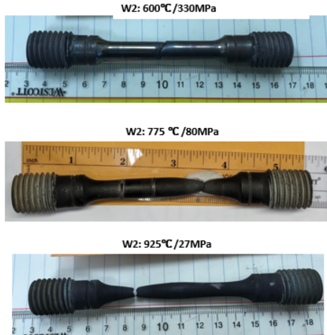
Figure 19. Photographs of the failed W2 weld specimens
