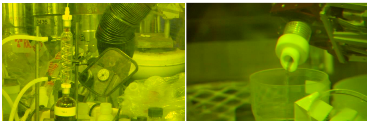
Figure 2. In-cell defueling apparatus (left) and filtration system (right).
