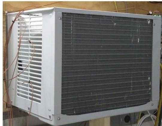
**Figure 14: Outdoor Side of WAC in Environmental Chambers**
