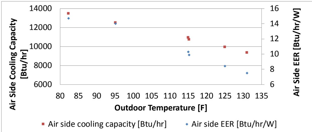
Figure 15: Measured air side cooling capacity and EER vs. outdoor air temperature
