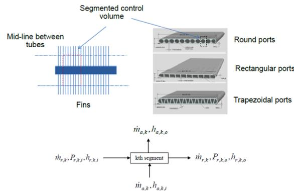
**Figure 9: Segmented Control Volume of a Mini-Port**
