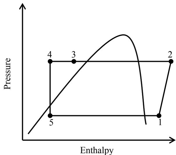
**Figure 2: P-h diagram of Window Air Conditioner**
