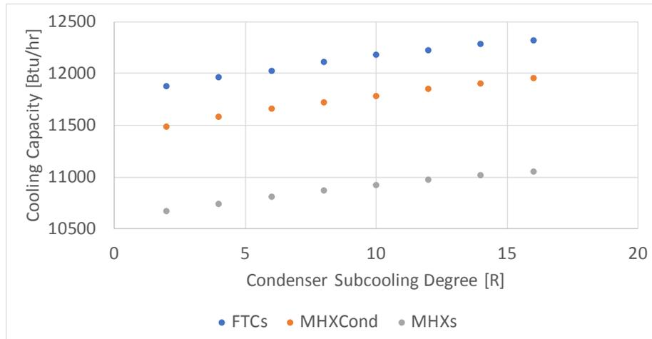
**Figure 18: Predicted cooling capacity as a function of the condenser subcooling degree**
