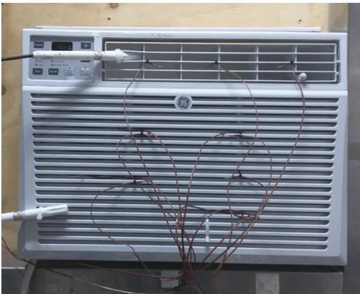
**Figure 13: Indoor Side of WAC in Environmental Chambers**
