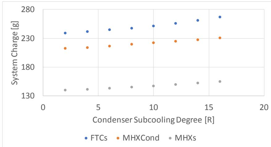
**Figure 16: Predicted system charge of R-290 as a function of the condenser subcooling degree**
