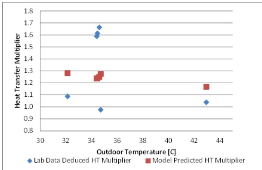
**Figure 10: Heat transfer enhancement ratio due to 'slinger effect' vs. outdoor temperature**
