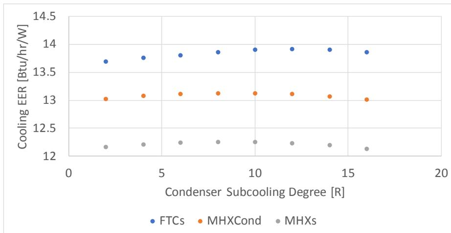
**Figure 17: Predicted cooling EER as a function of the condenser subcooling degree**
