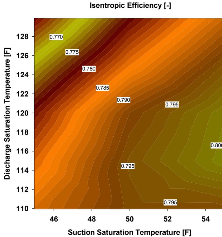
**Figure 11: Isentropic Efficiency Map of R-290 Sample Compressor**
