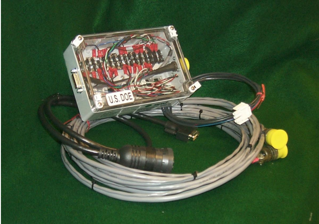
Figure 2. DASIB and associated cables.
