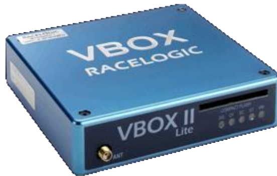
Figure 3. VBOX II Lite GPS unit.
